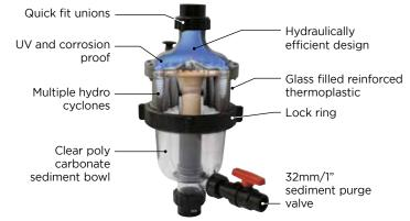
Incoming water enters hydro-cyclones tangentially, generating a strong centrifugal effect. The sediment is spun out to the hydro-cyclone's wall, and then spirals down to the sediment chamber. The filtered water migrates towards the centre of the hydro cyclone where
