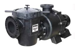
**Hydrostar Plus 1450 pumps are** high-performance corrosionresistant thermoplastic pumps equipped with a 6" flanged inlet port and 4" flanged outlet port. The pump's 4 pole motor runs at 1450 rpm making them ideal for high water flow applications such as aquatic facilities, water parks and large commercial swimming pools.
