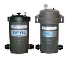
Opal cartridge filters are designed to house an extra large filter cartridge, maximising its dirt holding capacity and minimising filter maintenance. The filter's ergonomic lid allows easy access to the filter cartridge for removal, cleaning and installation in a matter of minutes.
