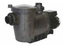
The Hydrostar MKIII has been redesigned to provide substantially quieter operation with even higher flow rates and higher head than the previous Hydrostar models. Waterco has improved the hydraulic efficiency of the pump with the introduction of an internal volute. The volute's hydraulic design provides a natural balanced water flow and reduces hydraulic turbulence.
