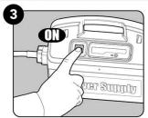
The robot will now begin working for a complete cleaning cycle. At the end of the cycle, it will automatically switch itself off
