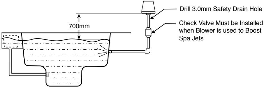
**b) AIR MANIFOLD INSTALLATION**
