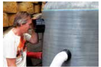
Generally, large manholes and sight glasses are harder to incorporate in high pressure filters, because any opening in a filter vessel creates a potential weak point or complicates the manufacturing process.
